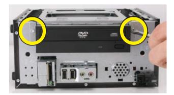
**12** Lift the front edge of the optical drive and cage assembly (1), and then slide the tabs (2) out of the notches at the rear of the computer.
